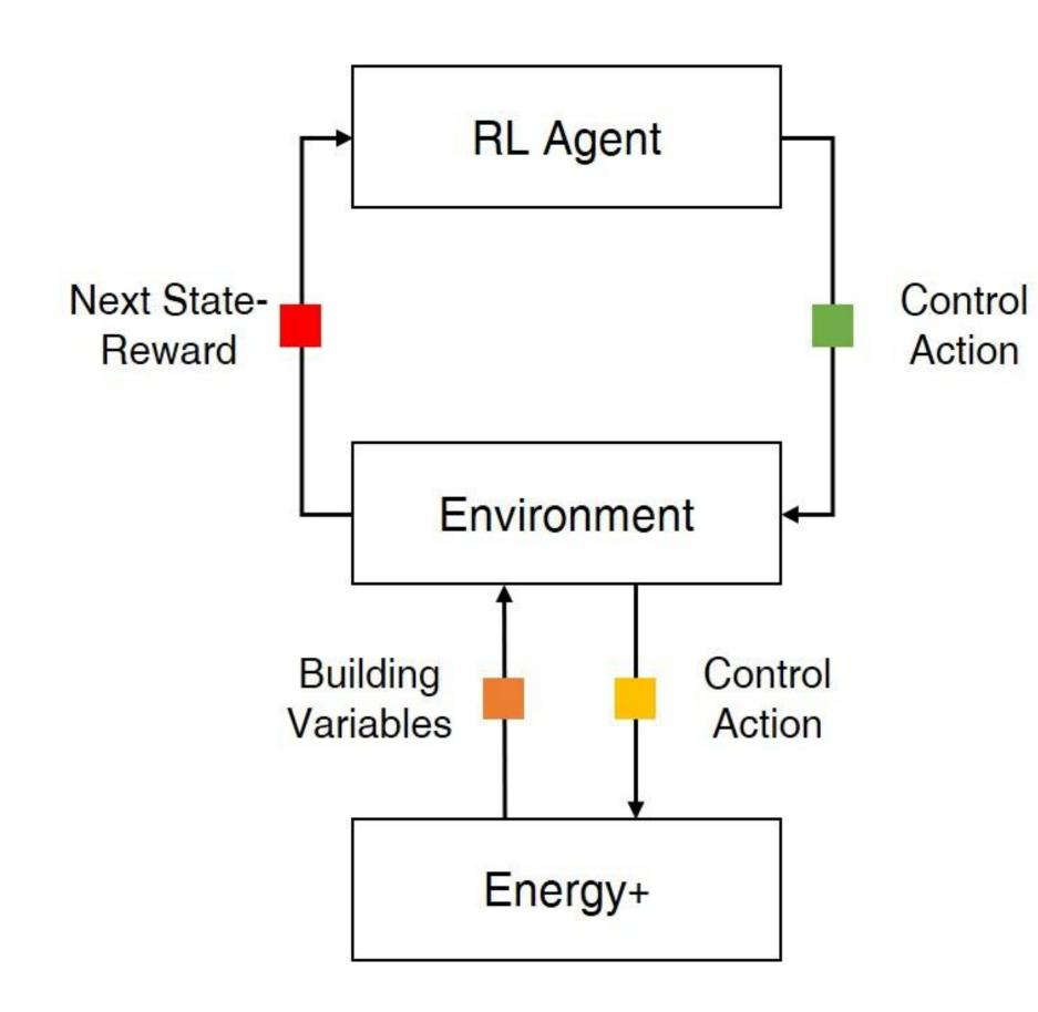
In the RL framework applied to HVAC control
